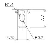
Solder Terminal (It can be used for TAB #187)
