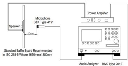
Test Conditions: Temperature: 15-30 ± 3°C Relative humidity: 25% ~ 80% Atmospheric pressure: 860 to 1060mbar
