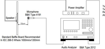
Test Conditions: Temperature: 15-30 ± 3°C Relative humidity: 25% ~ 80% Atmospheric pressure: 860 to 1060mbar
